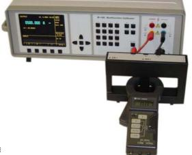
Current Coil Option 140-50 for calibration of clamp amperemeters.
